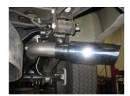
8. Install stainless steel tip. Clamp down. When you have everything in place, firmly tighten all bolts and clamps down securely. Inspect all fasteners after 25-50 miles of operation and re-tighten as necessary.
