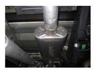
4. Install muffler #B onto headpipe #A 1.5-2" with louvers facing towards the converter. Use a jack stand to support the muffler
